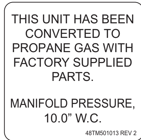
Fig. 7 - Propane Conversion Label – Propane Only
