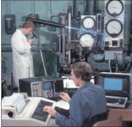
High-intensity illumination and fiber optic borescope enables research scientists to view valve action in compressor while it is running.
