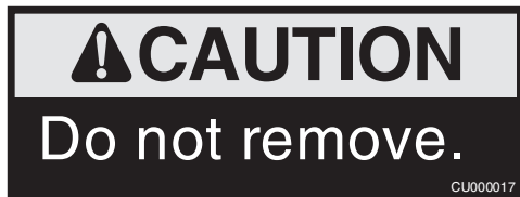
Fig. 3 — Panel Removal Warning Sticker — to be Placed on External Side of Cooling Coil Section Top Panel
