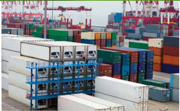
Refrigerated containers, stacked closely hundreds at a time on ships and thousands at a time in shipyards, require noncombustible refrigerants.
